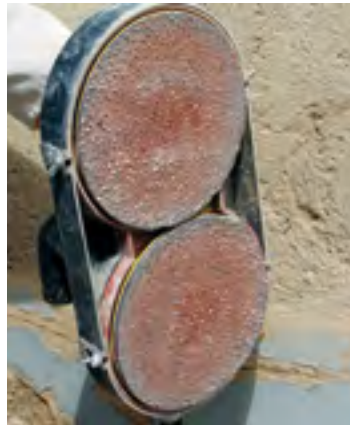
Removing old plasters
